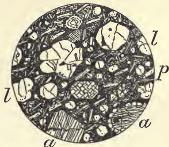
Fig. 40.—Leucite-Basalt. Vesuvius. \times 12 . a , Augite, in one instance surrounded by small leucites. l , Leucite; two large crystals lie in the upper part of the field. p , Plagioclase, associated with small leucites in the dark glassy groundmass.
